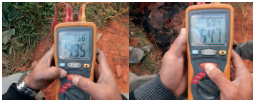
Figure 40 : Measuring Earth Resistance
